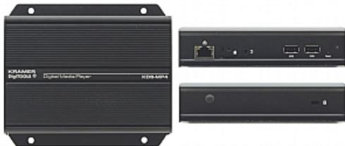
KDS-MP4 is a high-quality LAN-based 4K@60Hz (4:2:0) digital signage media player. The unit receives content from the Media Manager software installed on the PC, either via LAN or from an external USB memory stick, loads it into its internal memory and then displays it with image quality of up to 4K60 4:2:0 via the HDMI output
